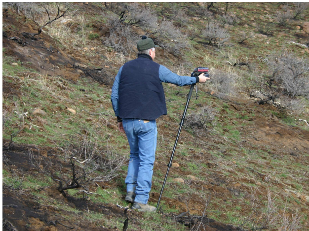
Figure 2. Acquisition of digital images in the field using a staff-mounted camera and a continuously recording GPS unit.
