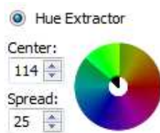
Figure 8. The Hue Extractor allows users to identify both the hue and the range used in classification.
