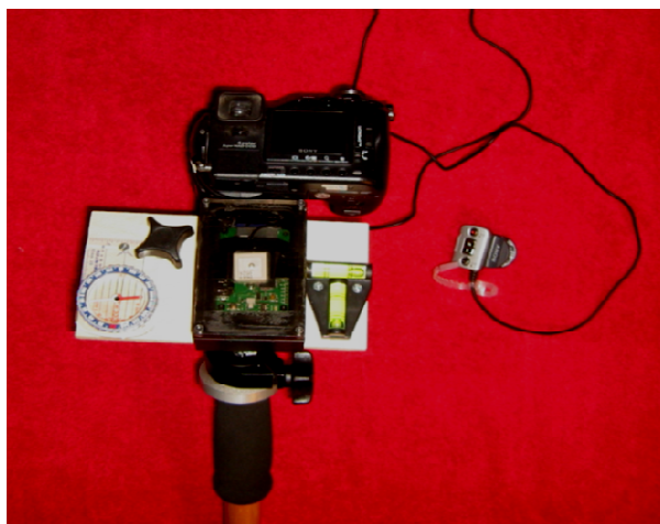
Figure 1. Apparatus used to obtain digital images of quadrats that are positioned with GeoAlbum software and classified using VegMeasure 2.
