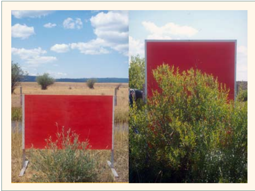
Figure 3. For field monitoring, we designed a lightweight photoboard constructed of an aluminum frame with a painted plastic board. For smaller willow clumps, the apparatus may be disassembled (left); the full board is used for larger clumps (right).
