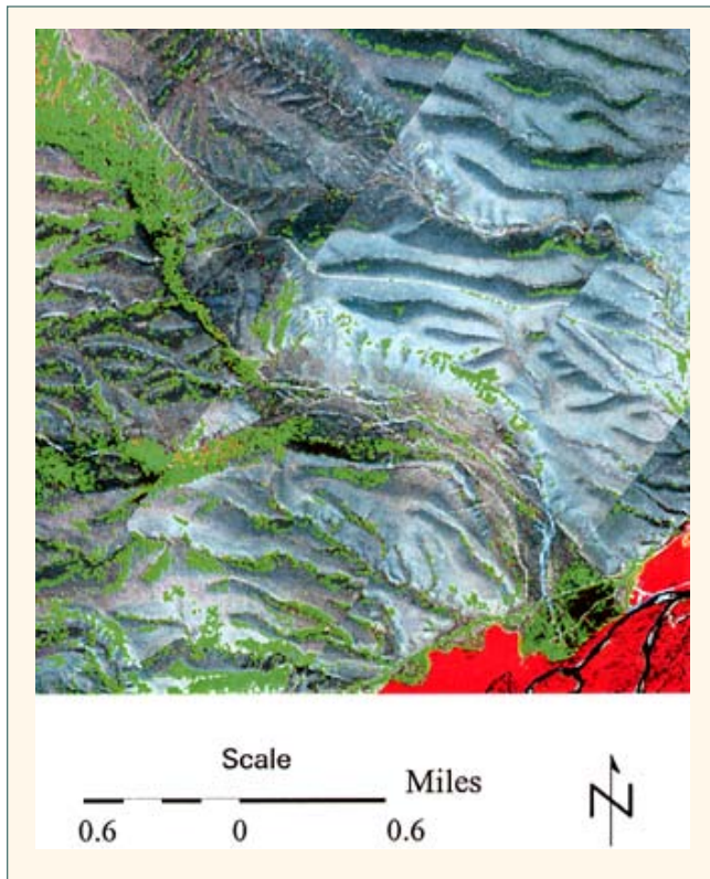
Figure 1. (Left) Classification of leafy spurge overlaid on hyperspectral imagery. Bands 24 (784 nm), 16 (662 nm), and 9 (555 nm) are displayed as red, green, and blue. (Right) Classification of spotted knapweed overlaid on hyperspectral imagery.
