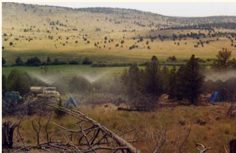
Figure 1. There were eight replications of cut and uncut plots. In every case the uncut plots experienced runoff and erosion. This picture shows the rainfall simulator application on cut (left) and woodland (right) treatments.
