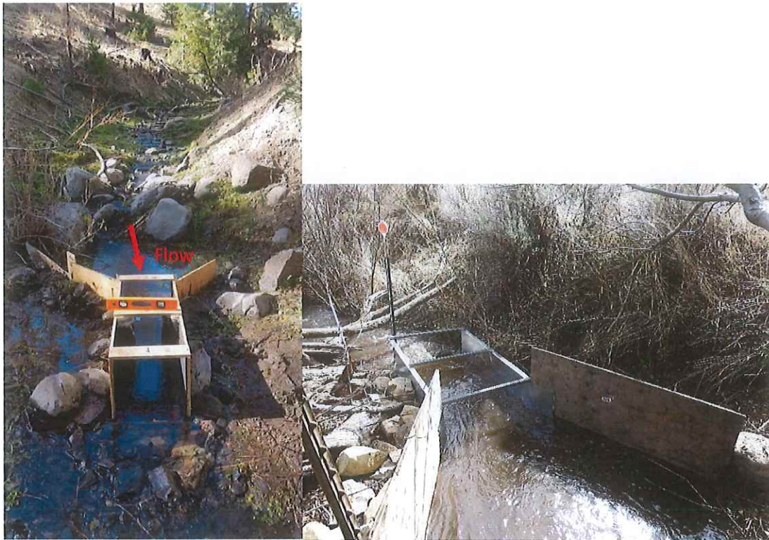
Streamflow measuring devices (above) installed and hourly streamflow at the watershed outlet (below). Streamflow was relatively low, peaking at 2.5 cubic feet per second (cfs) in April of 2021, following snowmelt runoff.
