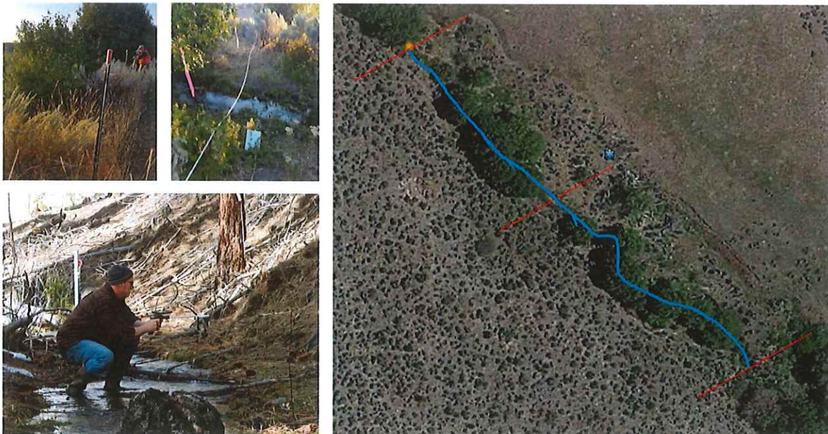
Figure 2. Schematic illustrating a 330-ft reach and methodology used to characterize stream morphology and riparian-upland vegetation. The line intercept method was used to determine cover along three 30-m transects perpendicular to the stream. Riparian area cover above the stream in the monitored reaches was collected using a canopy imager.
